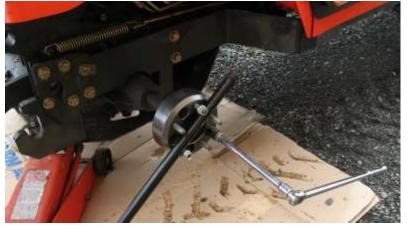
H. Get your socket & add Loctite to the studs on the spacer.
